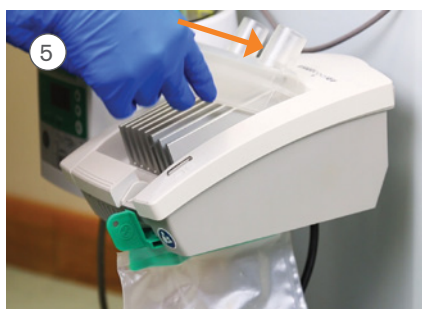
Insert the InterCooler cassette ensuring that the rear edge is located beneath the lip in the InterCooler base
