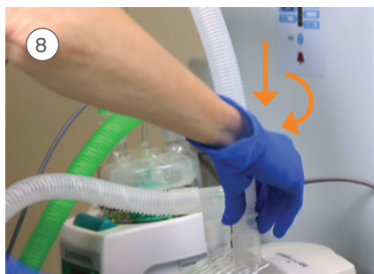
Connect the return limb to the 22mm female cassette connector
