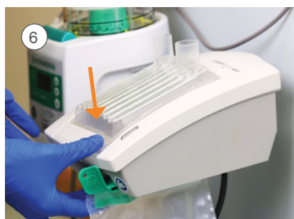
Push the cassette down and the latch forward , ensure location by checking that the latch is flush with the front of the InterCooler housing (see fig.1 over the page)
