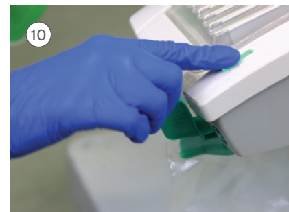
Turn on the InterCooler by pressing the power button . The button will illuminate green if the system is set up and functioning correctly
