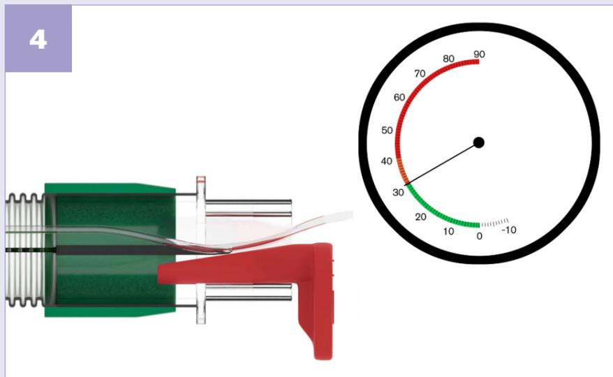
4 Pressurise the expiratory limb to 30cm H<sub>2</sub>O and confirm that there is no leak or pressure decay.
