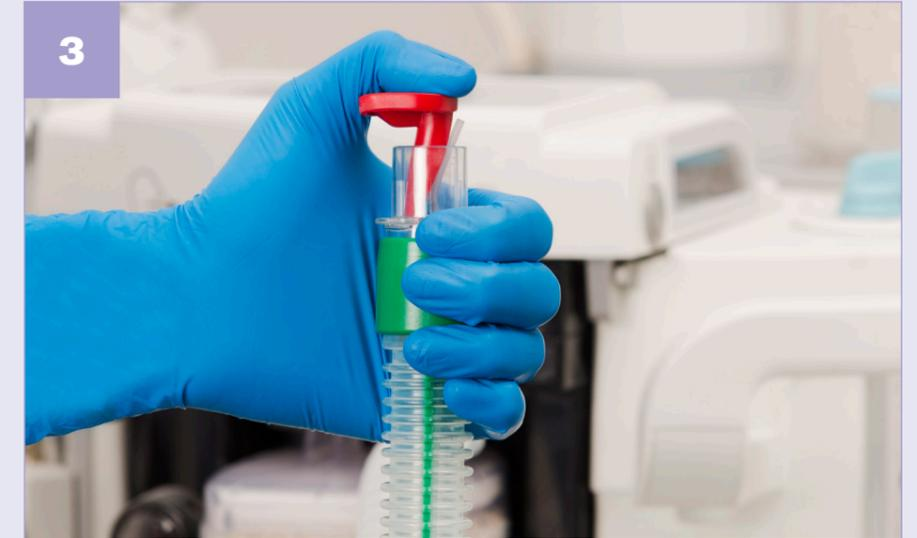
3 Occlude the expiratory side of the breathing system at the patient end using the supplied leak tester tool.
